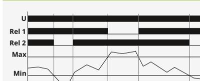
If the measured value falls below the adjusted MIN threshold, the output relay Rel2 switches into off-position. The output relay Rel2 switches into on-position again, as soon as the measured value exceeds the adjusted MIN threshold. If the measured value exceeds the adjusted MAX threshold, the output relay Rel1 switches into off-position. The output relay Rel1 switches into on-position again, as soon as the measured value exceeds the adjusted MIN threshold.
