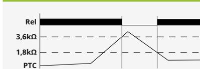
If the supply voltage U is applied and the cumulative resistance of the PTC-circuit is less than 3.6kΩ (standard temperature of the motor), the output relay R switches into on-position. When the cumulative resistance of the PTC-circuit exceeds 3.6kΩ, the output relay switches into off-position. The output relay switches into on-position again after the cumulative resistance falls below 1.6kΩ.
