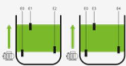
Pump up between probes E1-E2 respectively E3-E4 (alternatively control by one probe at a time). This feature allows level control in two separate containers with only one device. It is also possible to control cascades.
