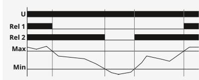
If the measured value falls below the adjusted MAX threshold, the output relay Rel1 switches into off-position. If the measured value falls below the adjusted MIN threshold, the output relay Rel2 switches into off-position. The output relays Rel1 and Rel2 switch into on-position again, as soon as the measured value exceeds the according adjusted threshold (MAX or MIN).
