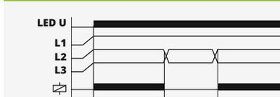
When all phases are connected in the correct sequence and the measured asymmetry is less than the fixed value, the output relay switches into on-position (yellow LED illuminated). When the phase sequence changes, the output relay switches into off-position (yellow LED not illuminated). It is recommended to connect the neutral wire of the monitoring relay once loads in the system use neutral connection.
