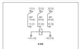
Note: the indicated polarity of the supply refers to the relays with extra equipment  ${\bf D}$  - surge suppression element (diode) - for DC coils only.
