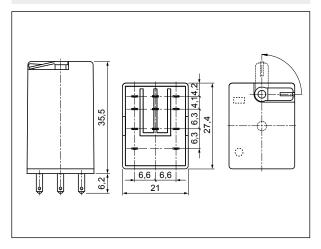
**Dimensions** - plug-in version, with test button (no latching) or with plug (no manual operation)
