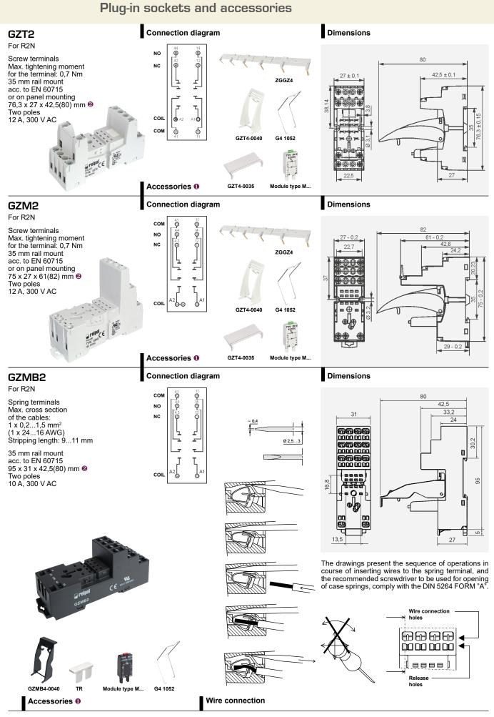
Mounting and sub-assemblies of accessories in the socket - see page 7. Signalling / protecting modules type M... - see page 9.
