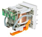
Application of electronics made in the SMD technology: additional features L (LED diode) and D (diode) are located on the printed circuit board; the change of the position of the LED diode and optimization of the quality and intensity of its light provide certainty that the relay is in operation status when the LED is on.
