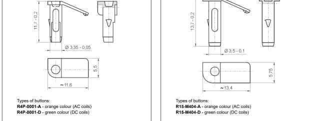
Plugs R4W-0003 or R15-M203 can substitute button type T if manual operation (latching and testing) is not allowed. Changing button type T for plug can be done by Customer themselves in the same way as changing button type T for button (no latching).
