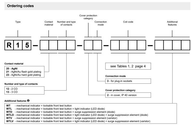
WT - standard features of relays for plug-in sockets. WTD, WTLD - only for DC coils, WTV, WTLV - only for AC coils
