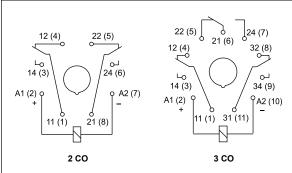
Note: the indicated polarity of the supply refers to the relays with extra equipment **D** - surge suppression element (diode) - for DC coils only.
