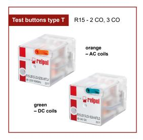
**Test buttons (no latching)** are recommended for R2N...WT, R3N...WT, R4N...WT, R15...WT 2 CO, R15...WT 3 CO relays - **for applications that do not allow permanent contact latching**. By manual operation (pressing the button) relay contacts can get switched for as long time as long the button is pressed. Contacts return to initial position as soon as pressure is released from the button. Those operations can be done while the coil is deenergized **6**.
