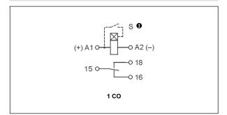
$\pmb{\theta}$  The control terminal S is activated by connection to A1 terminal via the external control contact S.
