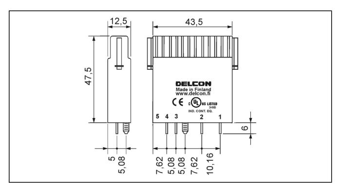
SLO-relay (plug-in), dimensions in mm.
