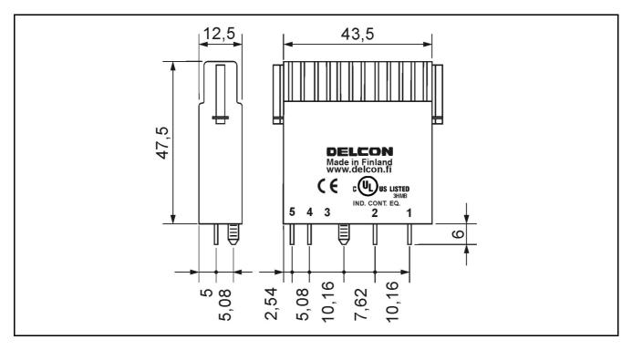
SLI-relay (plug-in), dimensions in mm.
