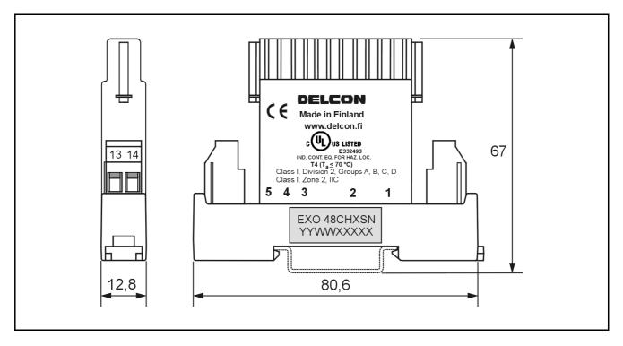
EXO 48CHXSN (dimensions in mm, nominal). Markings can be located differently by production lot. Parts of the markings are backside of the relay. Production lot number is marked to the socket (YY = year, WW = week, XXXXX = lot number).
