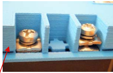
M4 control connection
