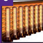
**Re-heat station by infra red heating lamps**
