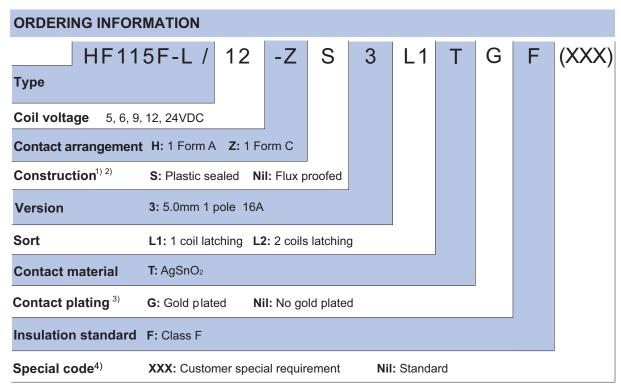
Notes: 1) We recommend flux proofed types for a clean environment (free from contaminations like H<sub>2</sub>S, SO<sub>2</sub>, NO<sub>2</sub>, dust, etc.). We suggest to choose plastic sealed types and validate it in real application for an unclean environment (with contaminations like H<sub>2</sub>S, SO<sub>2</sub>, NO<sub>2</sub>, dust, etc.).
