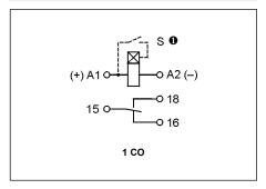
**1** The control terminal S is activated by connection to A1 terminal via the external control contact S.
